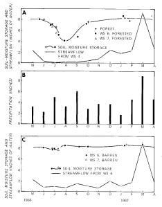
Figure 4.—Soil moisture-streamflow relationships. A, soil moisture in forest soil with discharge from a forested watershed. B, precipitation. C, soil moisture and streamflow from a barren watershed.
