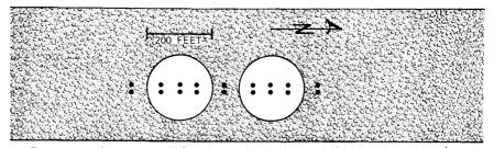
Figure 1.—Diagram of the access tube transect for comparing soilmoisture depletion in clearcut openings and in adjacent forest. The dots indicate positions of access tubes.
